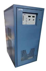
High Power Series range regulated and variable DC power supplies are solid state units utilizing thyristor technology in a single and three phase full-bridge rectifier topology that offer constant voltage control, constant current control, automatic crossover, series regulation, DC filter, digital metering and various operational and protective monitoring features.
