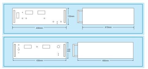
The New HIGH VOLTAGE DC Series offers a range of Regulated Supplies for use in Industries, PIV, HV, etc Research Labs, Capacitor Testing. The range has seven models. All the models have electrically floating outputs and operate in constant voltage current limiting mode.
